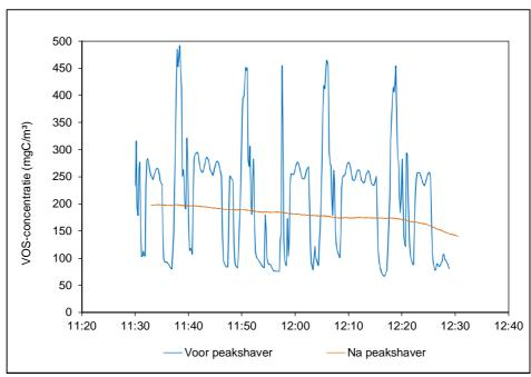
Figure 1. Effect of a peakshaver in front of a biological waste gas treatment unit (case: toluene at a spray booth)
