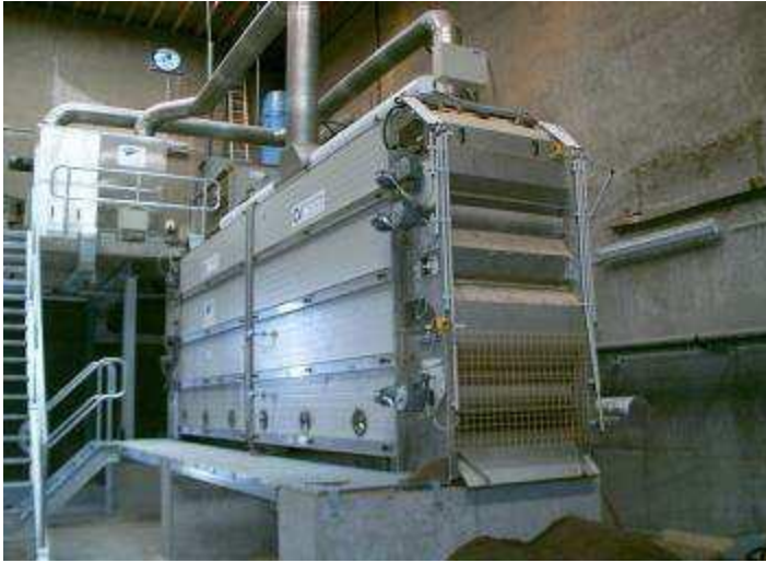
Picture 3. Condensation drier with drying unit in front and heat-exchanging unit on top
