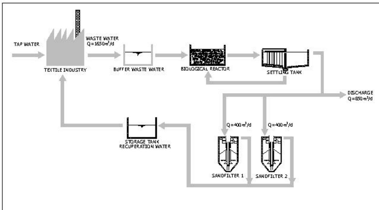
*Figure 2. Principle flow diagram recuperation unit in textile industry*
